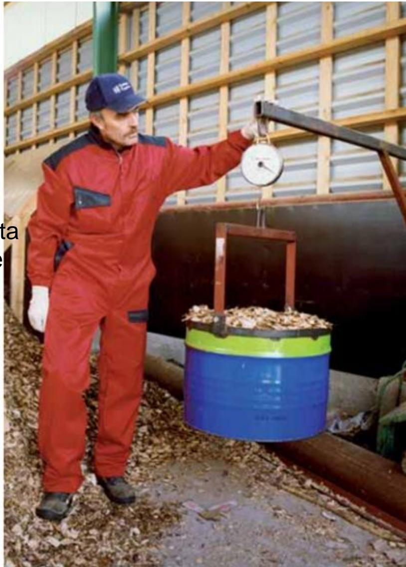
*Measuring bulk density. Photo: VTT*
