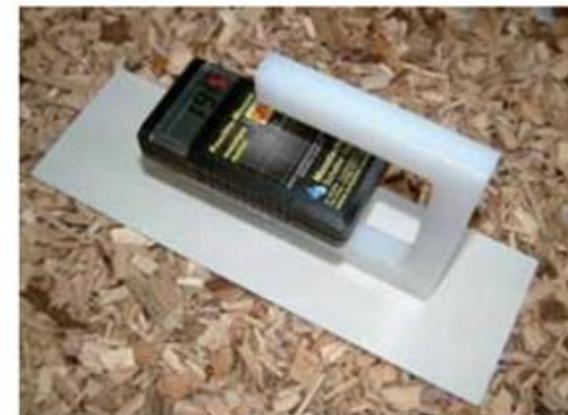
*Automatic measurement of the moisture content of the fuel. Photo: FJ-BLT*
